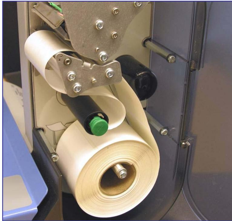
For stripped label operation, install the label roll on the supply spool and remove about 6 inches of labels from the liner. Slide the labels in the guides as shown.
