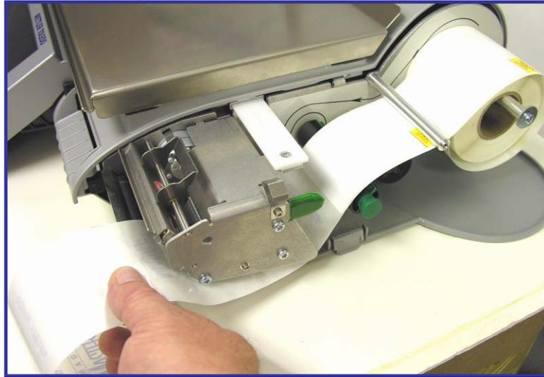
Install the label roll on the supply spool and remove about 6 inches of labels from the liner. Slide the labels under the guides and printhead as shown in the illustration.
