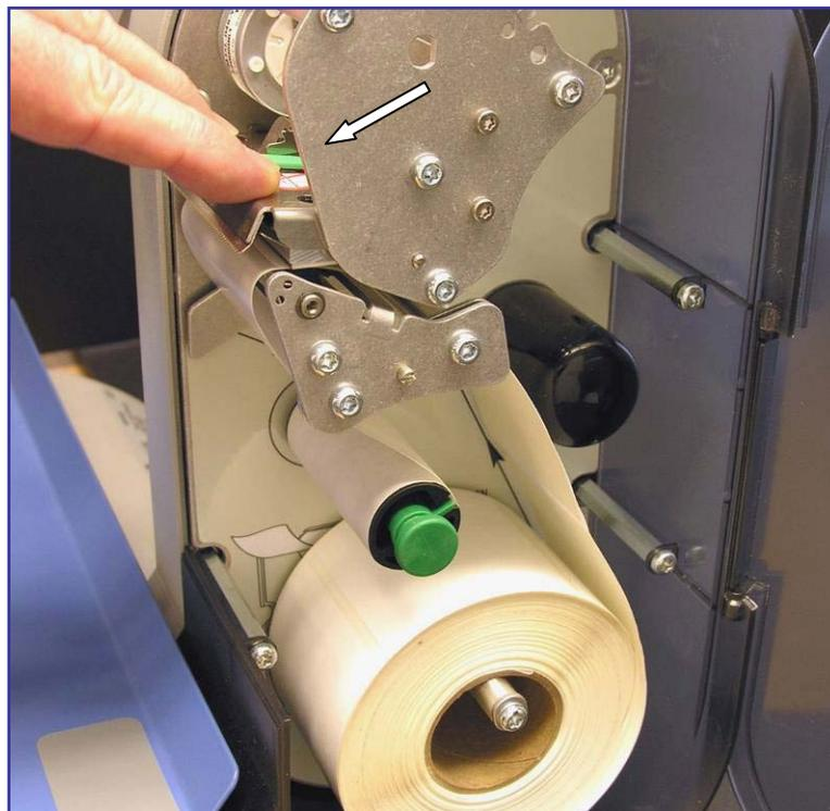
Press down on the printhead latch until it locks down.
