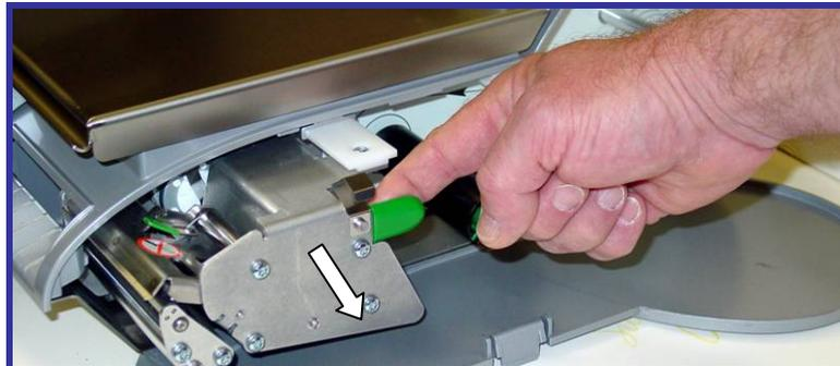
Pull the printer out using the green pull-tab on the printer.
