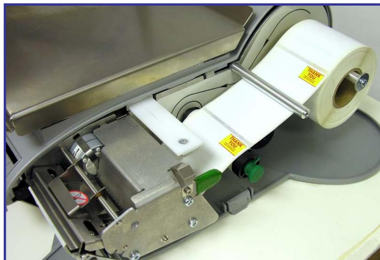
Shown is the printer with properly installed labels.
