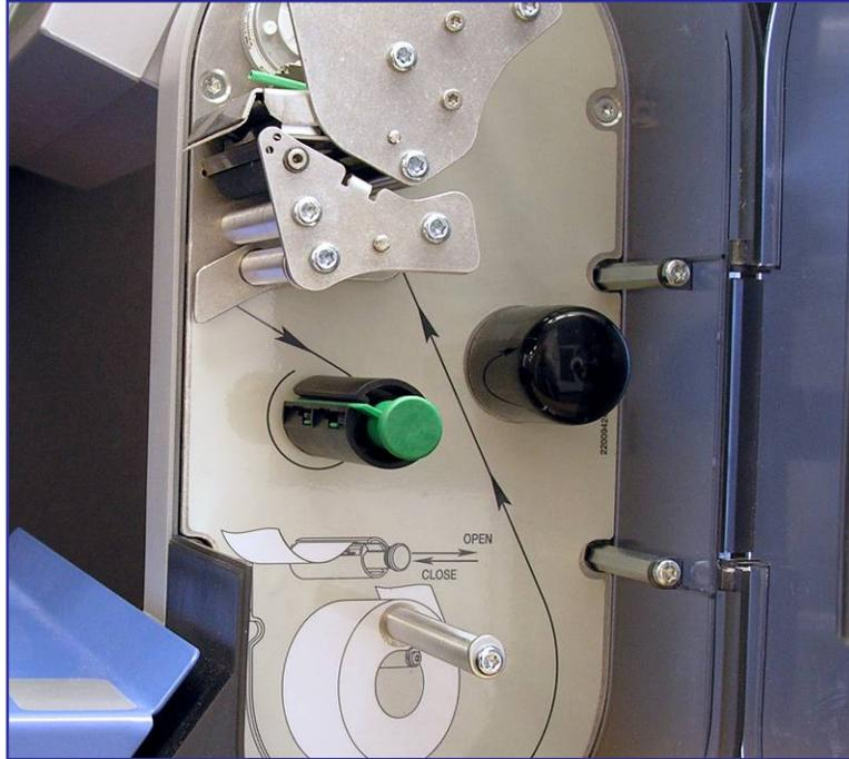
Open the printer door and refer to the label threading diagram backplate on the printer for reference in loading labels.
